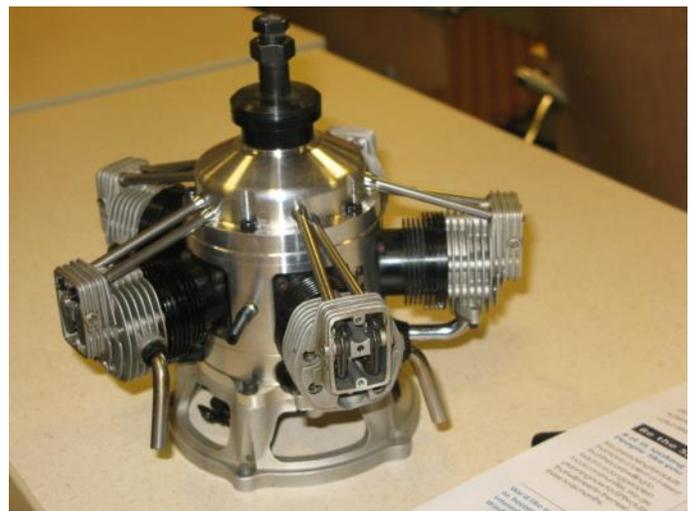
After extensive cleaning and rebuilding by Rikk, this radial is a pretty impressive engine
